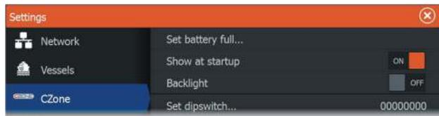
In order to communicate with the CZone modules connected to the network, the unit must be assigned a unique CZone Display Dipswitch setting.
